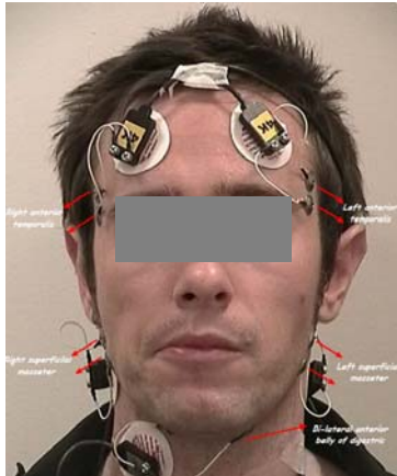
Figure 3. Experimental set up of surface electromyography, where electrodes were attached to target facial muscles to record their activities during an eating cycle.
