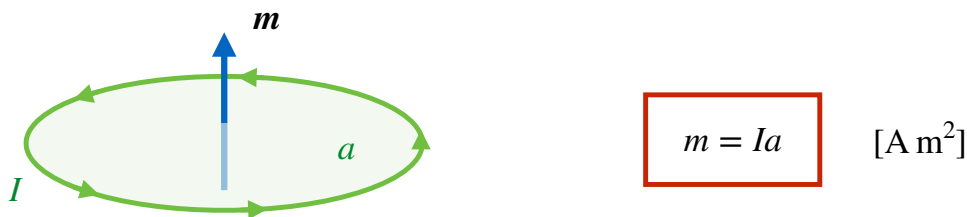
Figure 2.3: Magnetic moment characterising a current loop.
