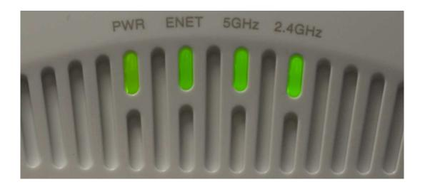
Green lights showing the presence of power (supplied over ethernet via a network switch capable of supplying 13W at a nominal 50V), wired ethernet activity (flickers), and that the two radios are working (b & g are 2.4GHz, a is 5GHz, n is both).
